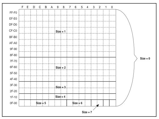
Figure 5-4. Address Range Allocation for Different Size Values
