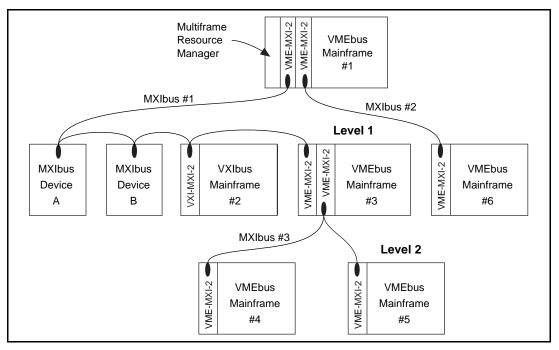
Figure 5-5. Example VMEbus/MXIbus System
