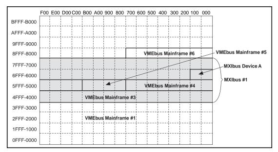
Figure 5-20. Example A16 Space Address Map Diagram
