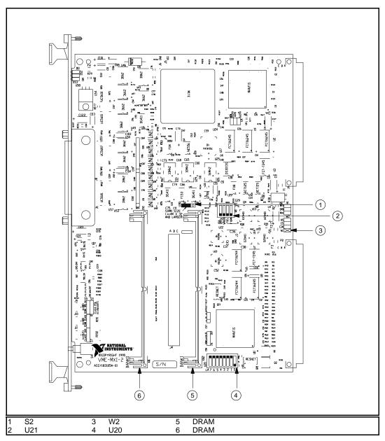
Figure 3-1. VME-MXI-2 Parts Locator Diagram
