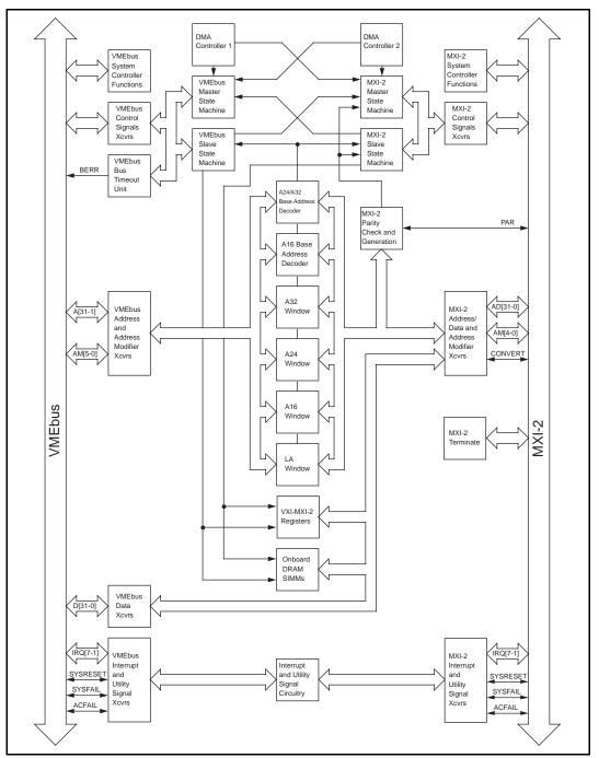
Figure 2-1. VME-MXI-2 Block Diagram
