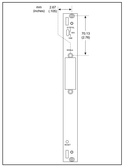
Figure C-1. VME-MXI-2 Front Panel Layout
