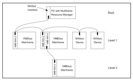
Figure 5-1. VMEbus/MXIbus System with Multiframe RM on a PC
