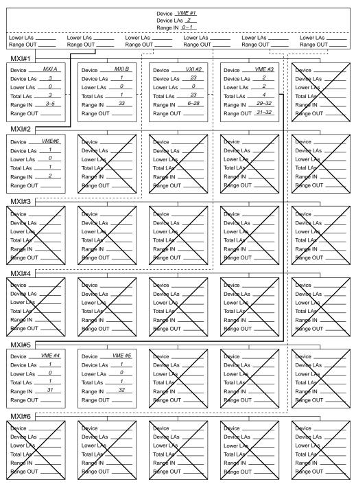
Figure 5-16. Alternative Worksheet: Logical Address Map for Example VMEbus/MXIbus System
