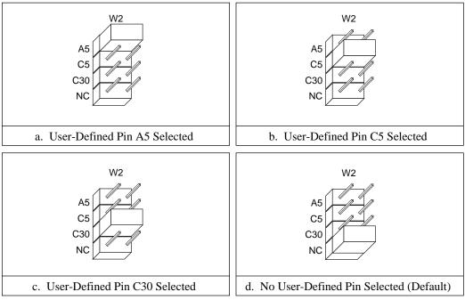
Figure 3-3. VME-MXI-2 Intermodule Signaling Settings
