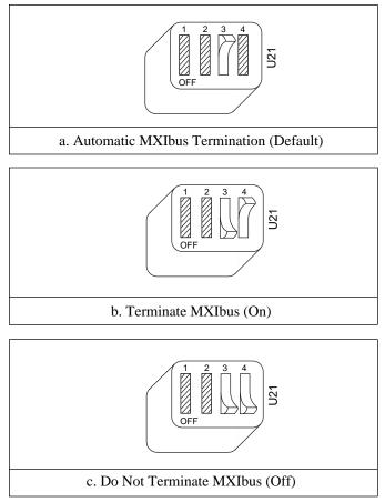
Figure 3-4. MXIbus Termination
