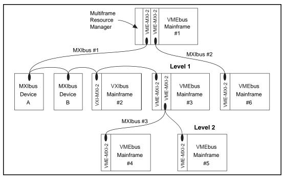
Figure 5-19. Example VMEbus/MXIbus System Diagram
